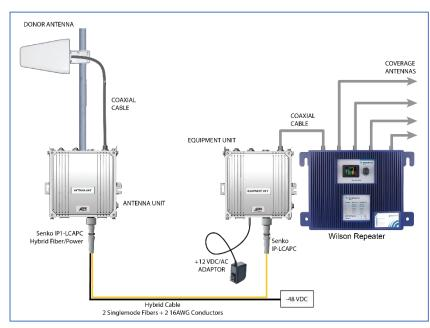
The Optical Zonu Antenna Extender provides an RF connection between the donor antenna and repeater when coaxial cable is not practical.
