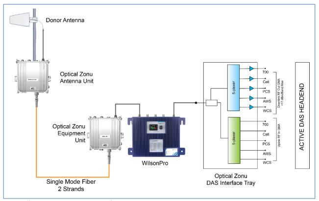
Case 2. Off-air connection to an active DAS. If the donor antenna is relatively close, the Antenna Extender would not be needed. The DAS Interface Tray splits the composite off-air signal from the WilsonPro into simplex, band-specification connections to the fiber DAS headend.
