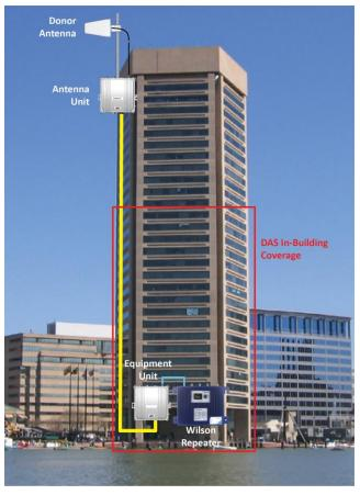
Case 1. Example of In-Building coverage for the lower floors of a high-rise. The repeater must be with the DAS on the lower floors but the donor antenna must be far away on the roof.
