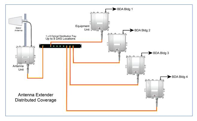
Case 3. Optical Zonu Distributed Antenna Extender. This configuration permits simulcasting of the off-air mobile wireless signals for up to 8 WilsonPro repeaters each driving a DAS in different buildings.
